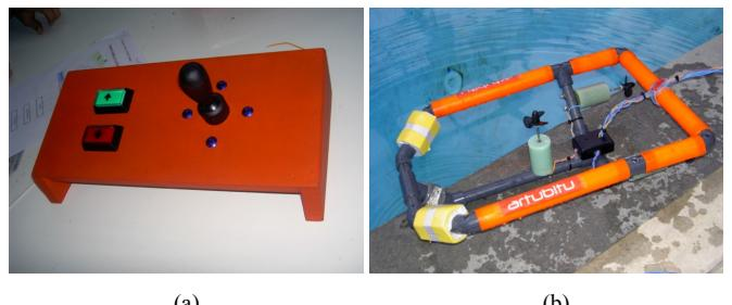
**Figure 3.** (a) Teleoperation unit or control console. (b) PVC chassis of a finished underwater robot.
