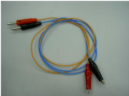
**Figure 4.** Testing wires equipped with alligator clips used to verify partial electric subsystems.
