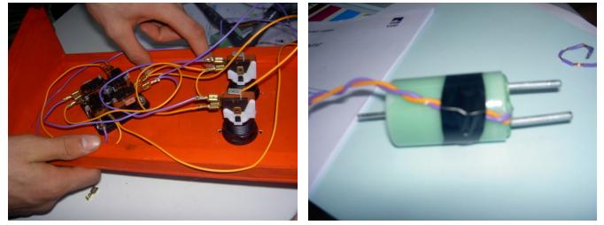
**Figure 5.** (a) Back side of the console: assembly of wire connections. (b) Wax sealed DC motor.
