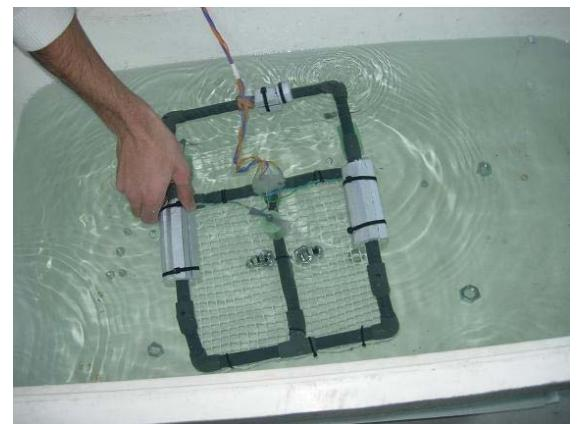
**Figure 7.** Small water tank for performing buoyancy and stability tests.
