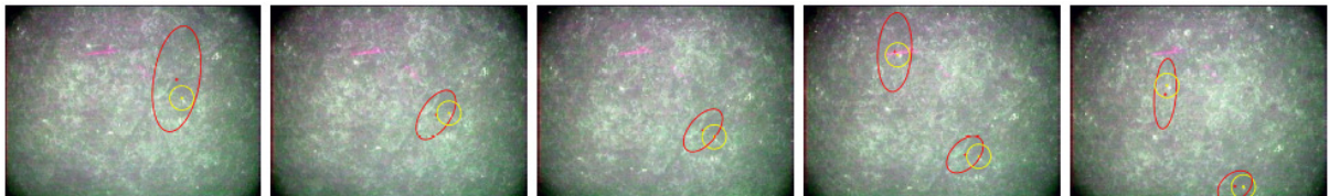
Fig.8: Sequence of down-looking camera frames. New observations and their associated measurement uncertainties are drawn, together with the prediction of a landmark that was already in the map, and the projection of its associated uncertainty onto the image plane. One can observe a reduction on uncertainty with new observations.
