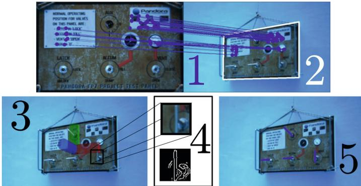
**Fig. 4.** Steps of the landmark detection: (1) Matching of keypoints between the template and camera image. (2) Estimation of the panel corners in the camera image. (3) Estimation of the template’s position and rotation in the image by using the camera parameters and the known geometry of the landmark. (4) Extraction of regions of interest and edges. (5) Estimation of valve orientation using Hough transform to detect lines from the edges.
