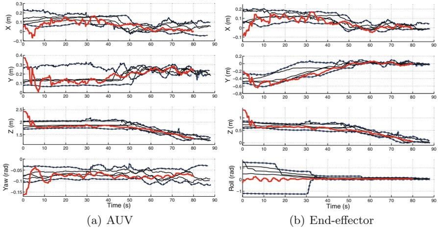
**Fig. 5.** Tele-operated trajectories (black) for the valve turning task, the upper and lower limit is depicted in dashed-blue and an autonomous trajectory is depicted in red. All trajectories are represented in the frame of the target valve. Each plot shows a single DoF for the AUV and the end-effector (Color figure online).
