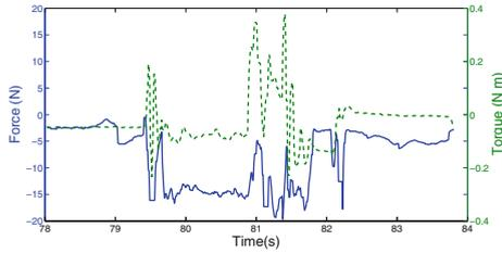
**Fig. 6.** Force and torque in Z axis measured in the end-effector during grasping and turning. It can be appreciated how a negative force was detected when touching the valve, and how the torque increased when operating the roll DOF (at second 81).
