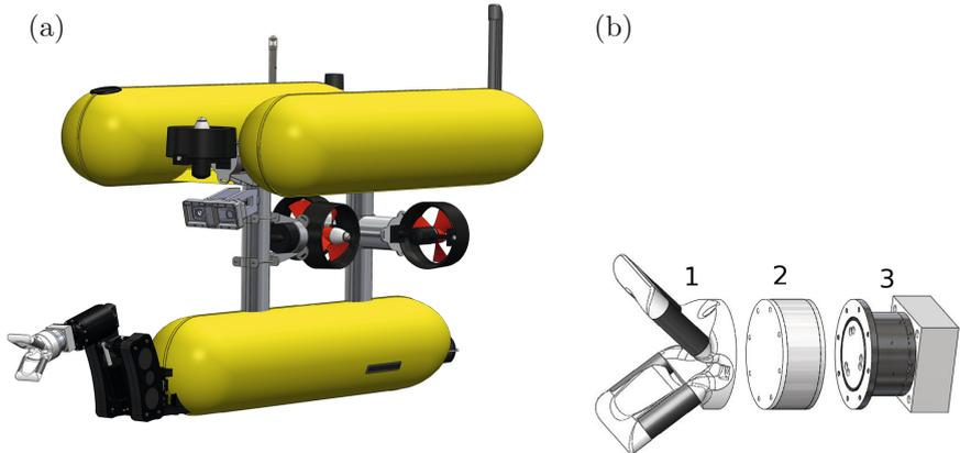
**Fig. 2.** (a) Girona 500 AUV with the 4 DOFs ECA manipulator equipped with a custom end-effector. (b) 3D model of the disassembled customized end-effector, in which three blocks can be distinguished: (1) passive gripper, (2) camera in-hand and (3) F/T sensor.
