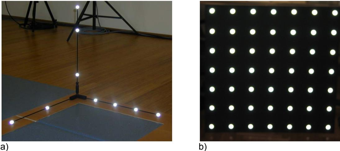
a) **Figure 1: a) Wand calibration: orthogonal triad of wands used for initialization of camera parameters and definition of spatial coordinate system; vertical wand (3 markers on) can be detached and used for a wand dance. b) 2D plate calibration: 7x7 coplanar calibration points.**
