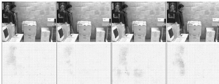
Figure 2. Example of Optical Flow: darker areas are the vectors of apparent velocities with length greater than zero
