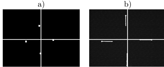
Figure 29: Experiment using a coarse alignment. a) Initial image. b) Final image with the trace of each laser point from its initial position to its final position.
