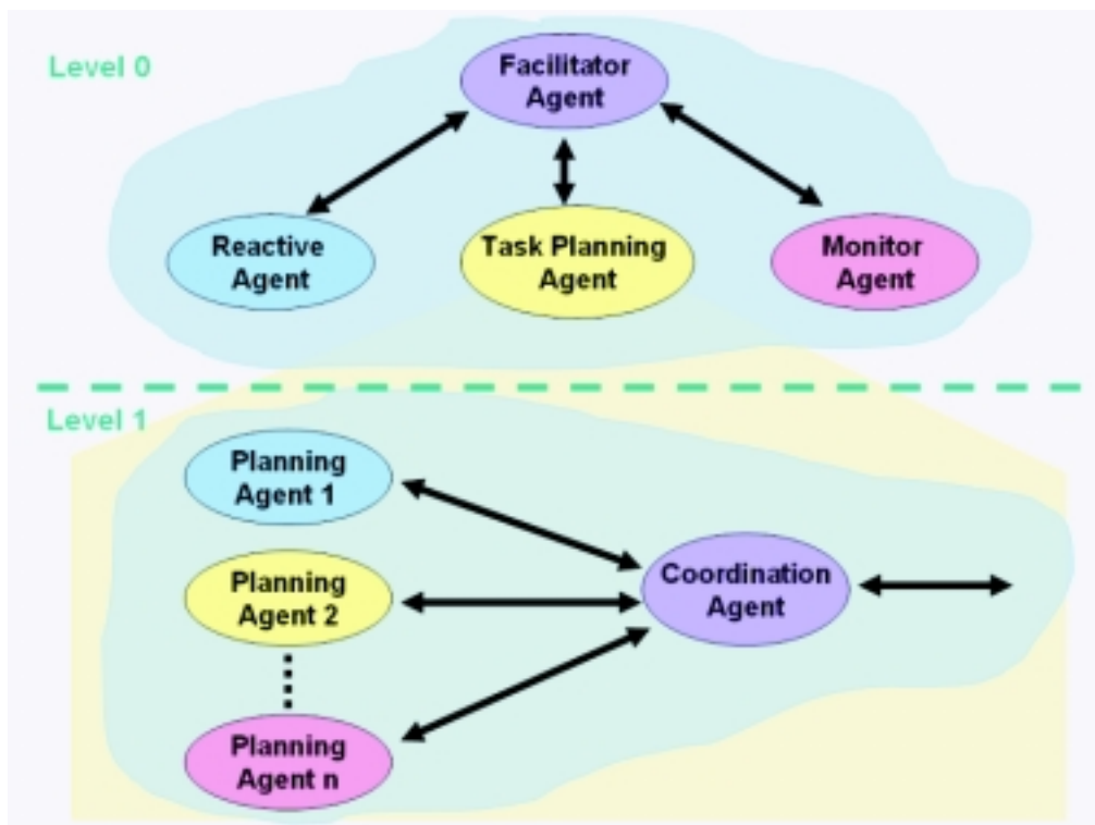
Fig. 1. The proposed MAS Architecture for Controlling a Mobile Robot. Level 0 is the most abstract level where agents may also be MAS. Level 1 shows the MAS subsystem corresponding to the Task Planning Agent (depicted in Level 0)
