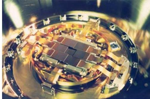
Figure 2.10: The CCD array of the camera incorporated in the XMM-Newton observatory (in orbit).
