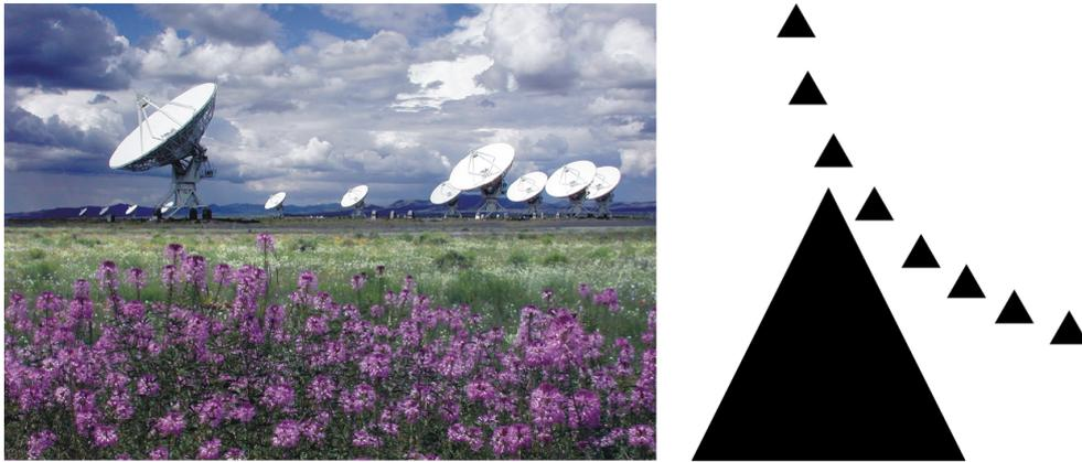
Figure 2.9: An example of an interferometer. On the left, the interferometer Very Large Array at USA. On the right, the diagram that shows the parabolic shape that aperture synthesis performs. Small triangles represent the set of radio antennas, while the big triangle represents the resulting big antenna that simulate the smaller ones.
